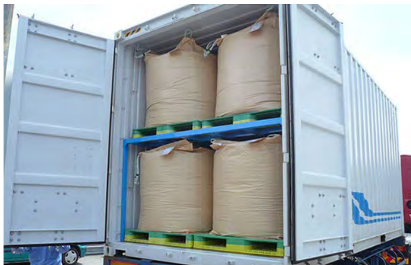
Dedicated racks enable FIBCs to be stacked
