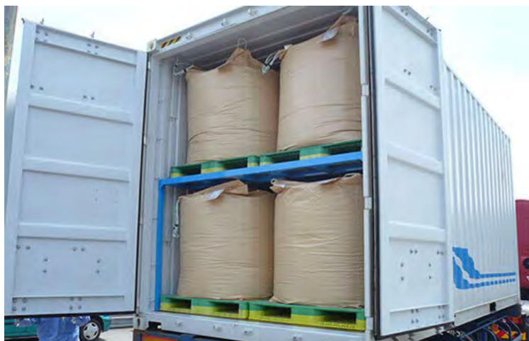
Dedicated racks enable FIBCs to be stacked
