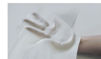
HUMOFIT™, a material that molds itself to fit human body at body temperature
