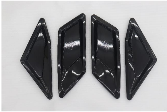
Hood air duct bezels (the direct pellet-fed 3D-printed components)
