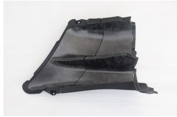
Decorative components on part of the front bumper (TAFNEX®CF/PP)
