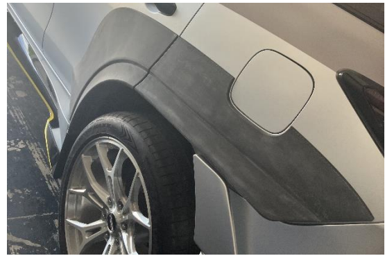
Rear overfender (direct pellet-fed 3D-printed components, before painting)
