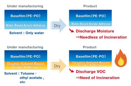
Reducing VOC and CO₂ emissions in Mitsui Masking Tape™ production process
