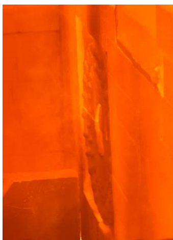
Figure 3. Flame during Ammonia Firing
