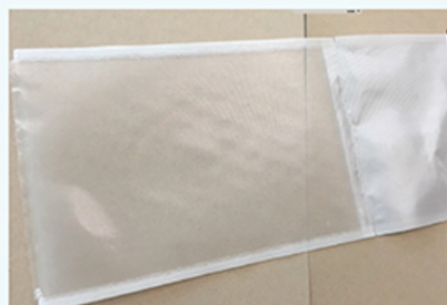
プリプレグ Prepreg (pre-polymer with glass cloth)
