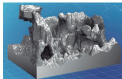
Integrated molding of an aluminum alloys joint and three CFRP structural material parts (left). Previously, these had been connected using screws, bushing, and other parts, with the components numbering 20. Above is an image of a metal surface after immersing in chemicals. Resin enters into the complex micropores and bonds tightly.
