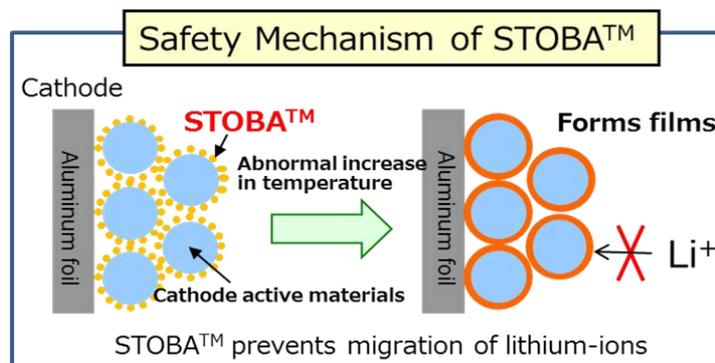
ITRI, Taiwan’s largest and leading R&D institution, developed this groundbreaking technology, with support from the Taiwan government, using nonconventional mechanisms and innovative materials to prevent thermal runaway of LIBs. In 2009, ITRI’s technology to enhance the safety of LIBs, STOBA<sup>TM</sup> (self-terminated oligomers with hyper-branched architecture) was recognized by R&D Magazine and awarded the “2009 R&D 100 Award in Energy Devices”.
