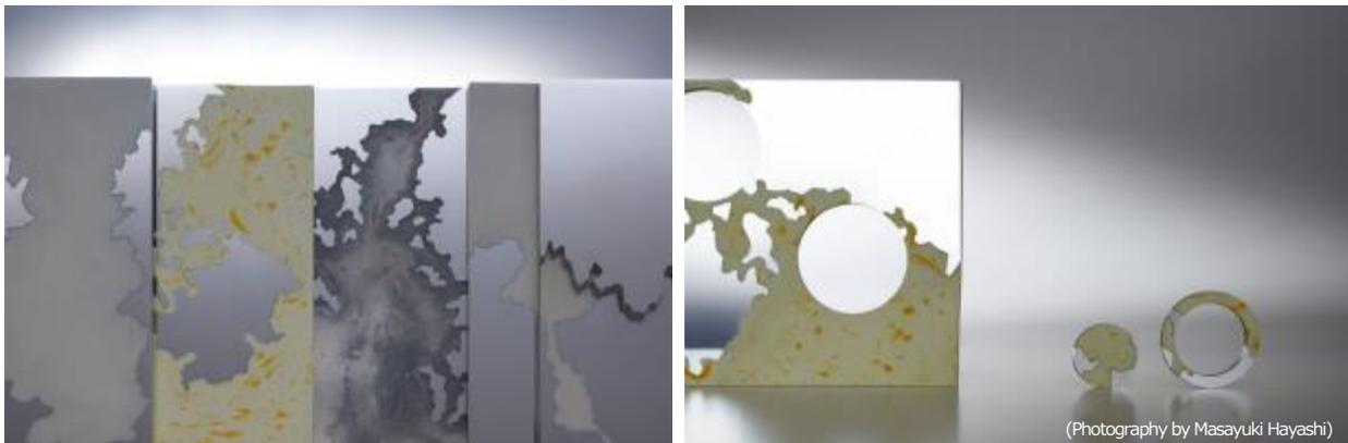
(Left) Plate material providing a macroscopic view of the bonding principle in POLYMETAC™ technology
