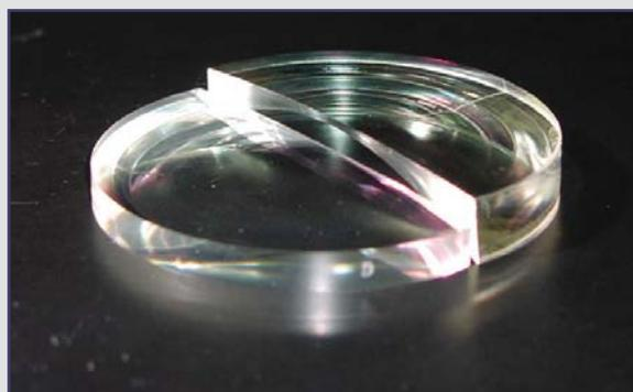
Thickness difference between MR Series (left) and 1.50 index lens (right)
