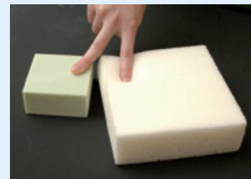
Two types of polyurethane foam with different level of hardness, which are made from castor oil.
