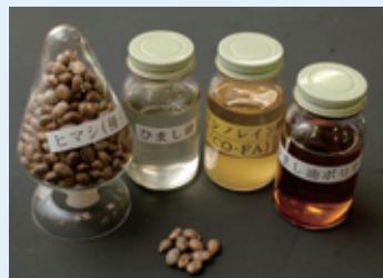
On the far left are castor seeds used as raw materials. To the right, castor oil is processed and refined into ricinoleic acid, which is used to make castor oil-based polyol, shown on the far right.
