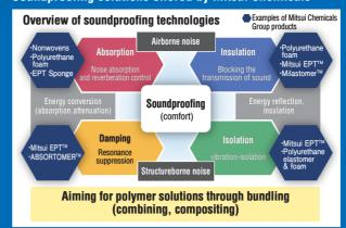
Soundproofing measures call for the analysis of how sound transmits and the setting of countermeasures. Sound absorption and insulation are effective against airborne noise, while damping and vibration isolation are effective against structureborne noise. Mitsui Chemicals has material technology suited to sound absorption, insulation, damping, and vibration isolation, and offers even more effective soundproofing solutions by combining these.
