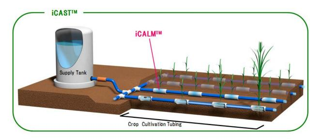
iCAST<sup>™</sup> is a unique crop cultivation system which supplies liquefied nutrients through tubes to a special planting bed using the proprietary material, iCALM<sup>™</sup> (integrated Cultivation-Accelerating Materials). As water, fertilizer, and pesticides are supplied through tubes to and retained in the iCALM<sup>™</sup> planting bed, crops can absorb nutrients and air as required (plant dependent growth factor delivery) resulting in optimal growth and quality.
