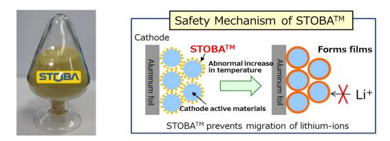
ITRI, Taiwan's largest and leading R&D institution, developed this groundbreaking technology, with support from the Taiwan government, using nonconventional mechanisms and innovative materials to prevent thermal runaway of LIBs. In 2009, ITRI's technology to enhance the safety of LIBs, STOBA<sup>™</sup> (self-terminated oligomers with hyper-branched architecture) was recognized by R&D Magazine and awarded the "2009 R&D 100 Award in Energy Devices".
