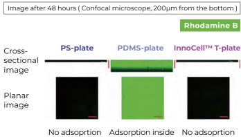
InnoCell™ T-plate is designed for and verified to have low drug adsorption into the culture substrate.
